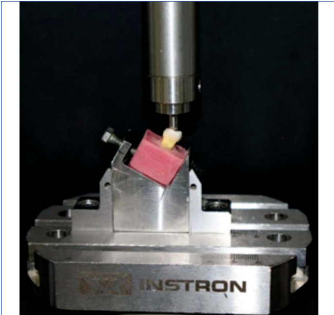
[Table/Fig-3]: Representative picture illustrating the failure endpoint used in the fracture resistance testing: the first audible crack accompanied by a visible structural fracture line at the site of load application.
